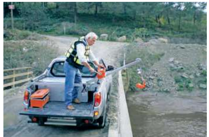
Car crane with Current Meter.
