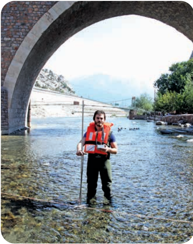
Measuring water velocity in the big river.
