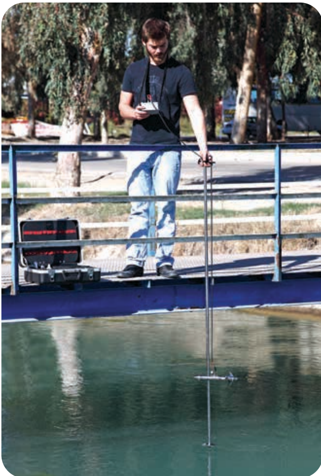
Measuring water velocity in the big channel
