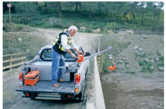
Car crane with Current Meter.
