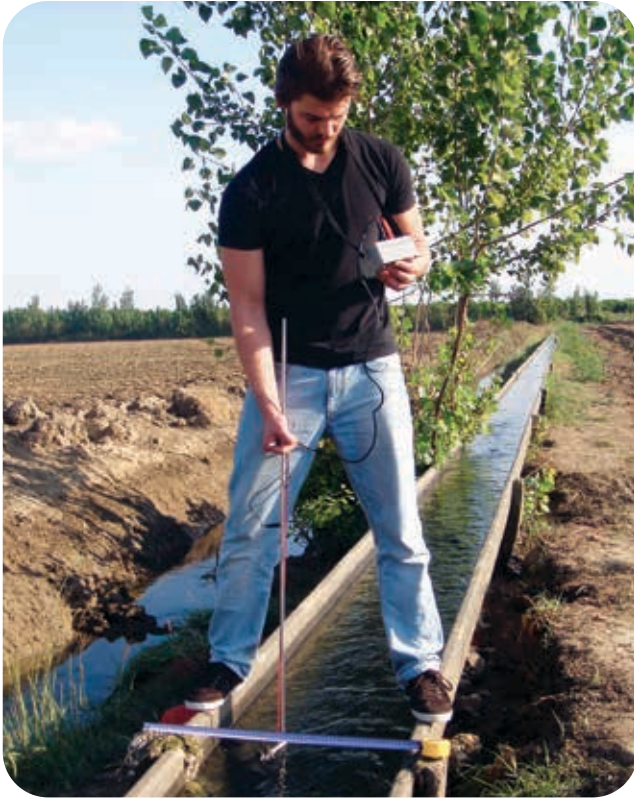
Measuring water velocity in the small canal.
