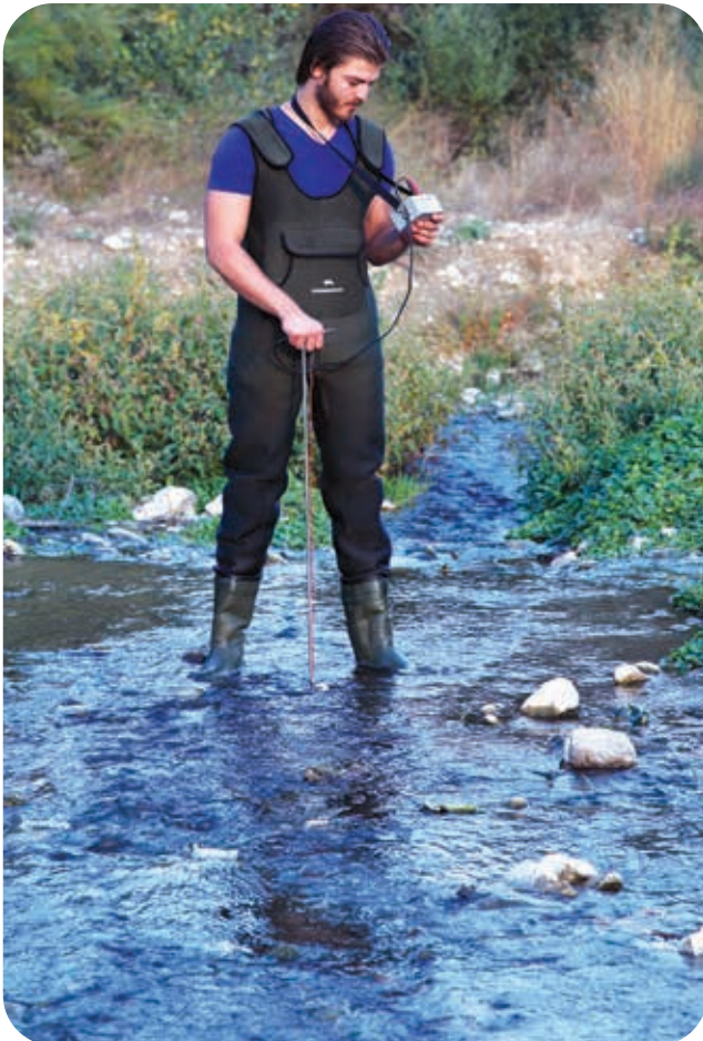
Measuring water velocity in the small river.
