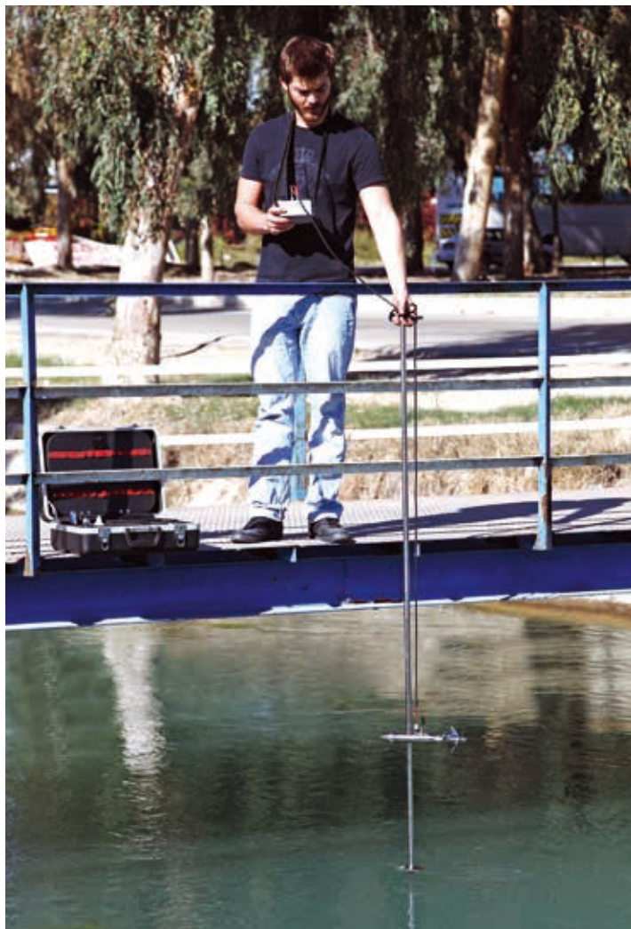
Measuring water velocity in the big canal.
