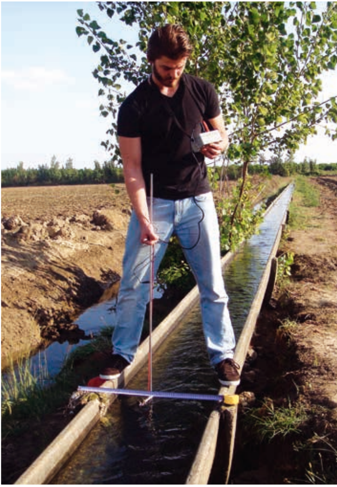
Measuring water velocity in the small canal.
